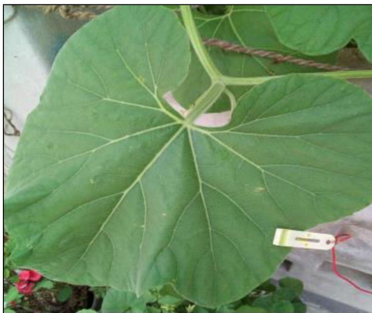
Fig. 1. Biosensor used for determining the moisture on the leaf.
